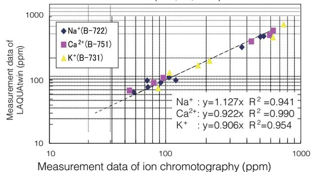
\*When measuring Ca<sup>2+</sup>, samples are pretreated in order to match the conditions of the ion chromatography.
