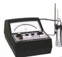
M-5 (benchtop) conversion from vacuum tube to semiconductor allows miniaturization and development of fast response meter
